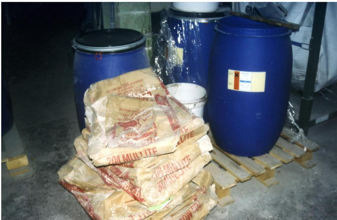
*Fig. 4: Dust source as a result of the storage of empty paper bags*
