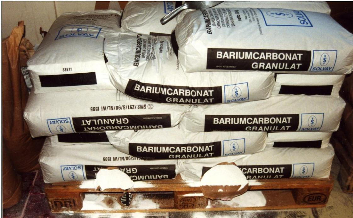
*Fig. 2: Barium carbonate sacks damaged by plant-internal traffic; the raw material is provided as granulate*
