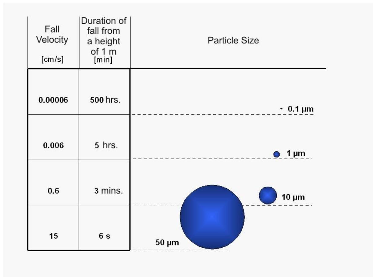
Fig. 1: Floating behaviour of dust particles (density 2 g/cm<sup>3</sup>) in air
